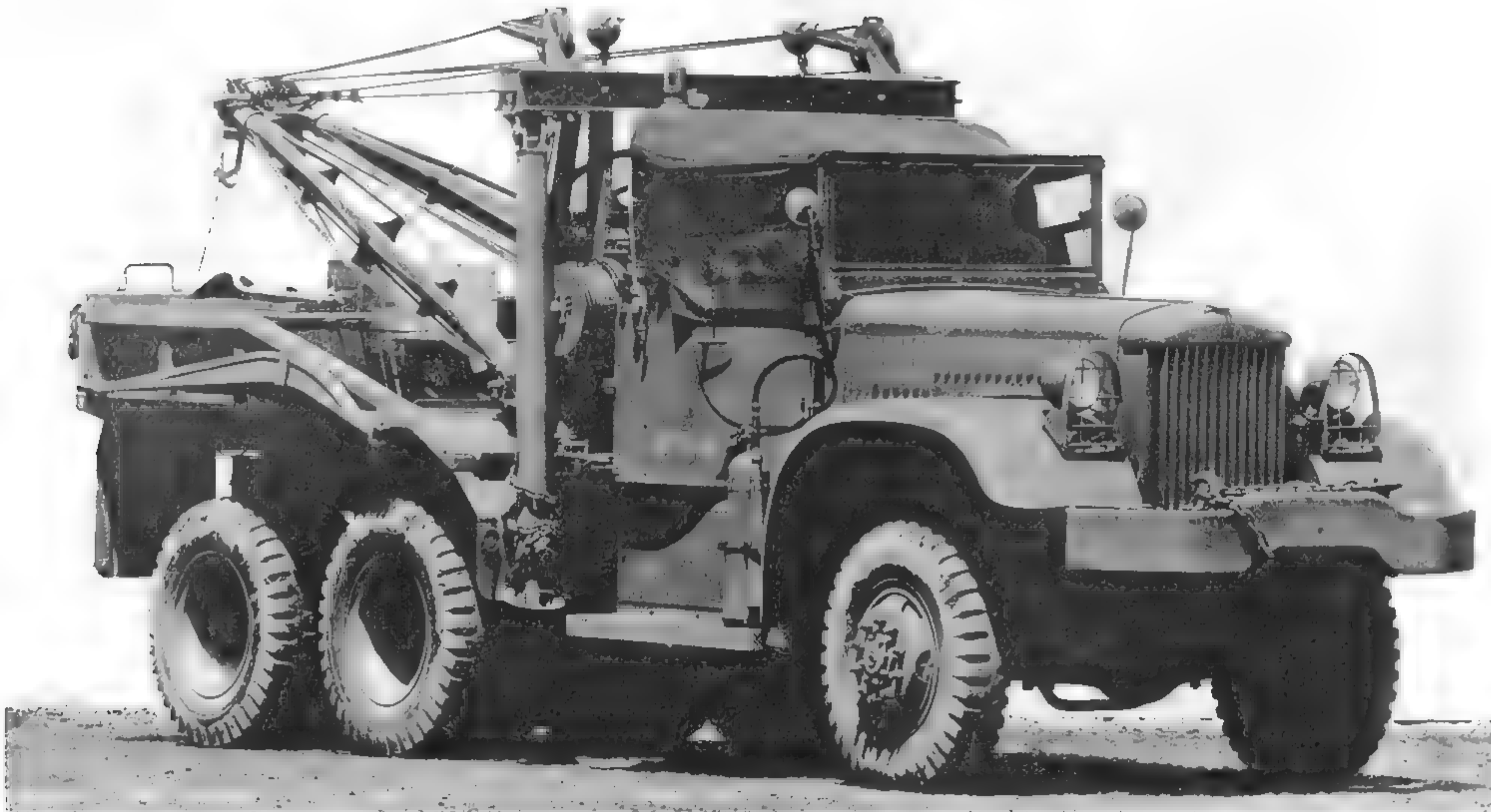
The last wreckers delivered had open cabs. The open-cab design was not adopted to save metal. It actually requires as much or more material as a closed cab. The chief benefit was better visibility of enemy aircraft for the crew. The tire tread is the more common non-directional type. The tires, regardless of tread design, were 9.00-20, 10-ply. (U.S. Army photo)
